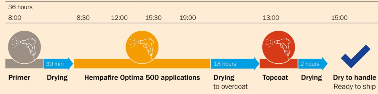
Primer applied, 3600 µm DFT of PFP, topcoated with PU and handled in 36 hours
