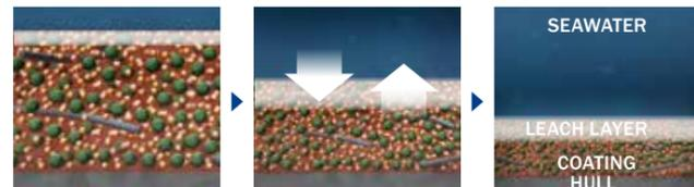
Seawater penetrates the coating and hydrates the rosin (yellow) and biocide (green). The rosin dissolves and the biocide leaches out of the coating. An insoluble 'hard' polymer structure remains, weakened in the absence of synthetic rosin, and is physically eroded by the ablative effect of surface water currents. Over time, the zinc carboxylate makes sure the leach layer remains low while releasing a controlled level of biocide.
