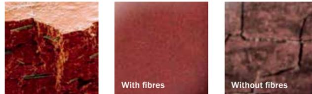
The microfibrils run close to the surface to ensure best-in-class mechanical strength.
