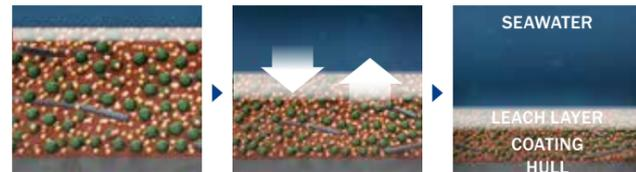
Seawater penetrates the coating and hydrates the rosin (yellow) and biocide (green). The rosin dissolves and the biocide leaches out of the coating. An insoluble 'hard' polymer structure remains, weakened in the absence of rosin, and is physically eroded by the ablative effect of surface water currents. Over time with steady rosin and biocide release, the leach layer becomes thicker. No coating remains at the end of the docking interval.
