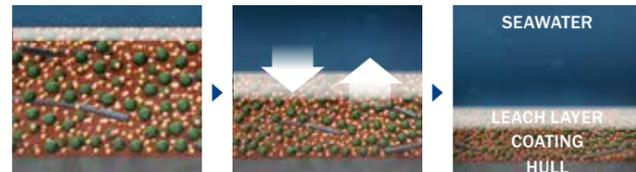
Seawater penetrates the coating and hydrates the rosin (yellow) and biocide (green), which dissolves and leaches out of the coating. An insoluble 'hard' polymer structure remains, weakened in the absence of rosin, and is physically eroded by the abrasive effect of surface water current. Over time with steady rosin and biocide release, the leach layer becomes thicker. At the end of the docking interval there will be no coating left.
