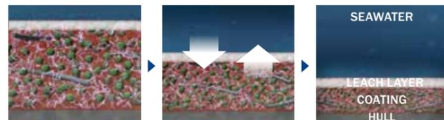
Seawater penetrates the outer layer, starting hydrolysis. As the level of hydrolysis rises, the polymer (light grey) starts to become soluble, forming a leach layer and releasing the biocide (green). The leach layer is progressively eroded from the surface, exposing a fresh coating layer underneath.
