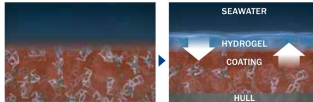
Upon immersion of the low-friction silicone coating, a hydrogel microlayer forms at the silicone-water interface, where it acts as a physical fouling defence. Actiguard technology enables controlled release of biocide via the active hydrogel micro layer. The biocide-activated hydrogel reinforces the fouling defence, significantly extending the fouling-free period and effectively improving fuel efficiency.
