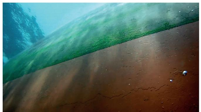
After 23 months of trading in warm and fouling-aggressive waters, the hull of the Famenne was inspected in the United Arab Emirates. The Hempaguard test patch was still exceptionally fouling free.
