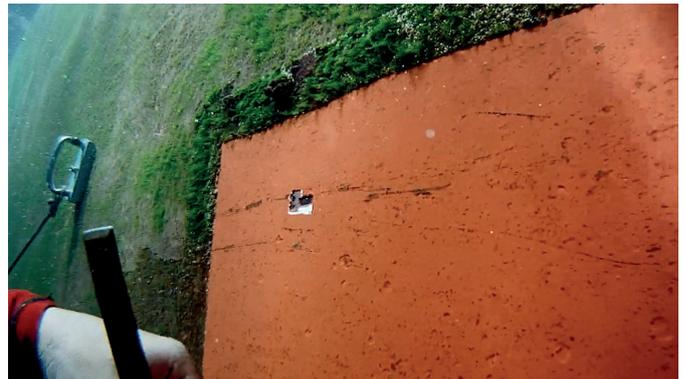
In comparison, the standard SPC antifouling coating suffered from heavy fouling. This high fouling build-up was largely due to relatively long idle periods during the test.
