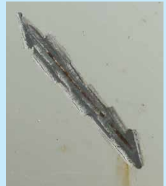
Full system with Avantguard technology (1440 hours)
