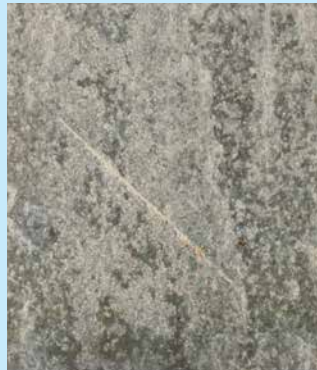
Zinc epoxy with Avantguard technology (986 hours)
