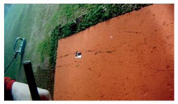
In comparison, the standard SPC antifouling coating suffered from heavy fouling. This high fouling build-up was largely due to relatively long idle periods during the test.
