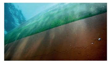
After 23 months of trading in warm and fouling-aggressive waters, the hull of the Famenne was inspected in the United Arab Emirates. The Hempaguard test patch was still exceptionally fouling free.
