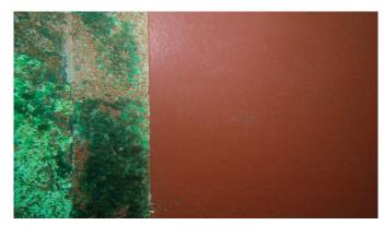
After 45 months, the Hempaguard test patch was inspected during a night dive in Singapore. The Hempaguard test patch was still smooth and fouling free. This 'remarkable' performance has convinced Euronav to complete full-scale Hempaguard applications on a number of vessels, starting with the Suezmax Devon.
