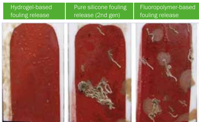
Figure 2: Comparison of static performance of 3 different Fouling Release technologies. The pictures have been taken after 8 months of static immersion in Singapore.
