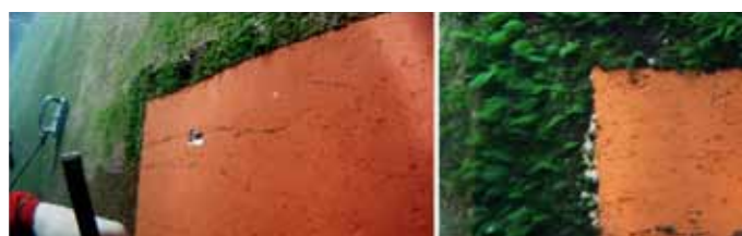
Figure 9: Pictures of a test patch after 22 months in service. The area on the pictures is scratched but still shows excellent performance.
