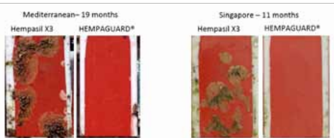
Figure 8: Pictures of panels damaged by sandpapering. Left: Hempasil X3 compared to Hempaguard after 19 months immersion in Spain. Right: Hempasil X3 compared to Hempaguard after 11 months immersion in Singapore.
