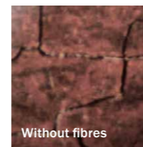
Coating condition after exposure to a cyclic blister box test: No failures were observed on the panel reinforced with microfibrils. The coating without microfibrils showed severe cracking.
