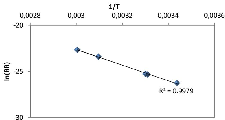
**Figure 9: Observed release-rate data from ActiGuard® coatings at different temperatures. The data is fitted to an Arrhenius plot.**
