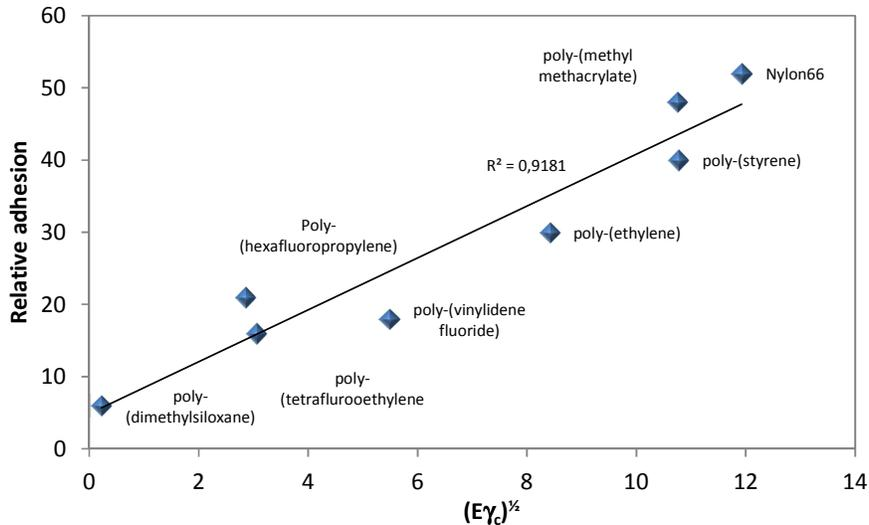
Figure 2: Relative adhesion as a function of squareroot of the product of the substrates elasticity and surface tension. Data from Brady and Singer [2000]
