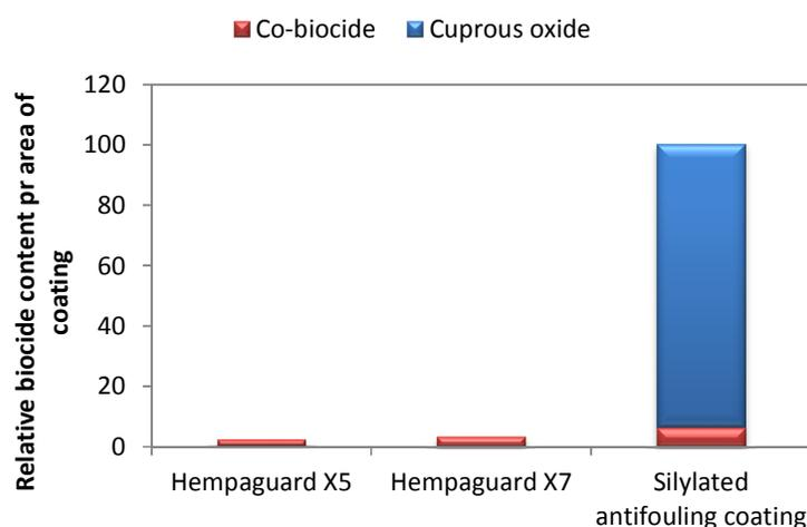
Figure 6: Average biocide release over the life-time of the coatings for HEMPAGUARD® X5 and X7 compared to a conventional silylacrylate antifouling coating. The calculation is based on conventional specifications (150 µm DFT for HEMPAGUARD® and 280 µm for the antifouling system).
