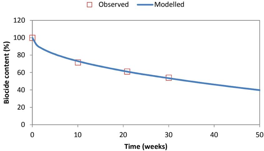
Figure 7: Model of biocide content over time in a dynamically immersed HEMPAGUARD® coating.
