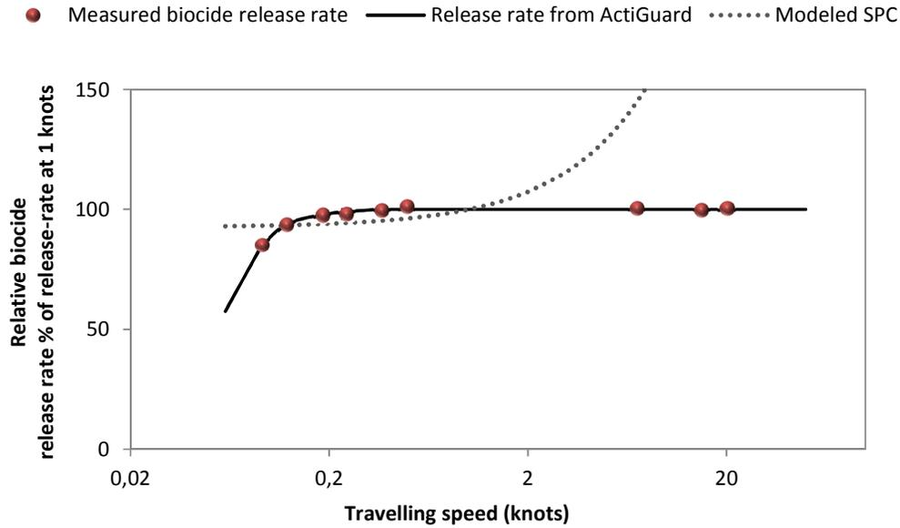
Figure 11: Relative biocide release rate from ActiGuard® as a function of travelling speed. Also indicated is the relative biocide release rate from conventional SPCs (adapted from Kiil et al. 2002). Note the logarithmic scale on the X-axis.
