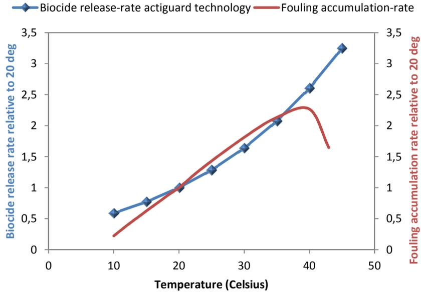
Figure 10: Comparison of development of biocide release-rate from ActiGuard® and fouling pressure as a function of temperature.
