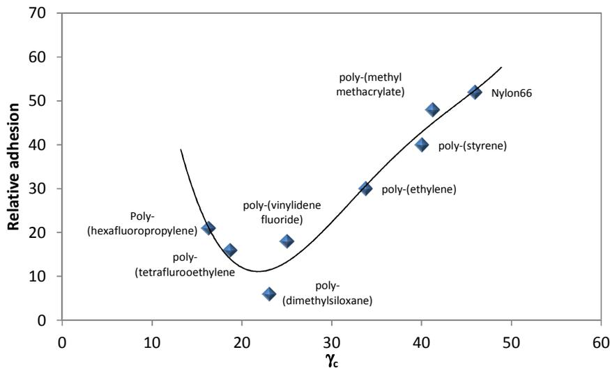
Figure 1: The 'Baier curve': Relative adhesion as a function of surface tension. Data from Brady and Singer [2000]
