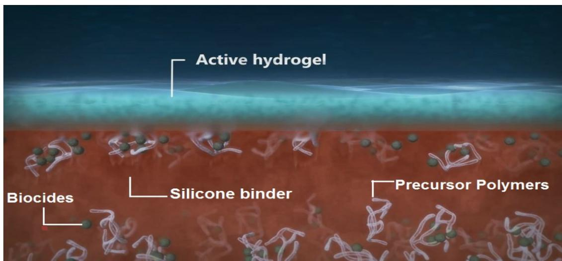
**Figure 5: schematic illustration of ActiGuard®.**
