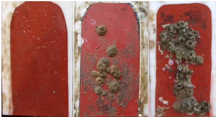
**Figure 4: comparison of biocide-free and biocide containing commercial Fouling Release coatings. Left: Hempasil X3 after 8 months immersion in Singapore. Middle: Hempasil 77500 with biocide after 7 months in Singapore. Right: Fluoropolymer Foul Release coating with biocide after 7 months in Singapore.**
