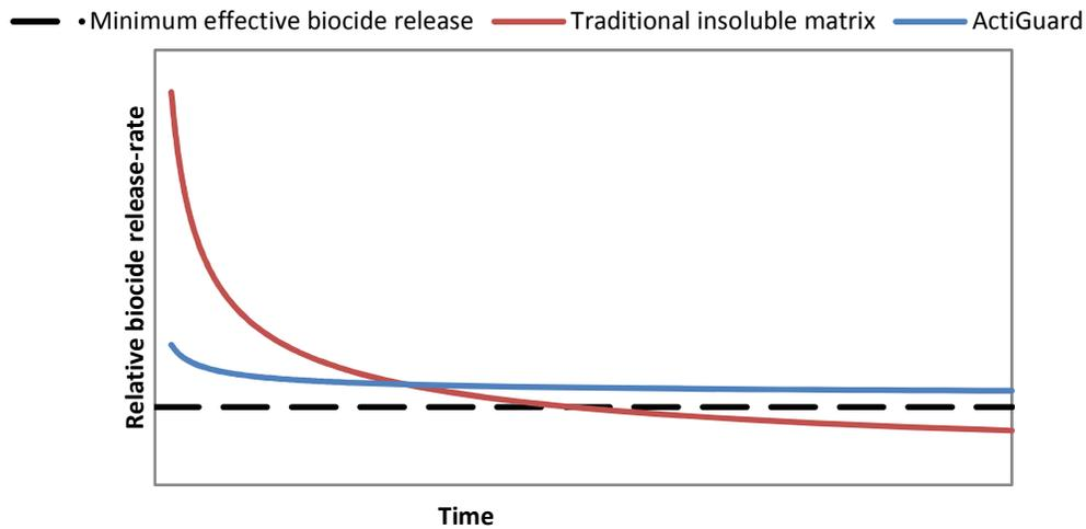
Figure 8: Comparison between the development in biocidal release-rate between ActiGuard®, and a conventional insoluble matrix antifouling coating. Both coatings contain a similar amount of biocide initially. A minimum effective biocide release-rate is indicated by a punctured line.
