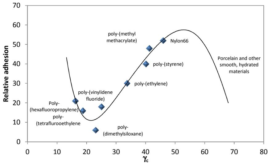
Figure 3: Relative adhesion as a function of critical surface tension. Modified from Baier [2006]
