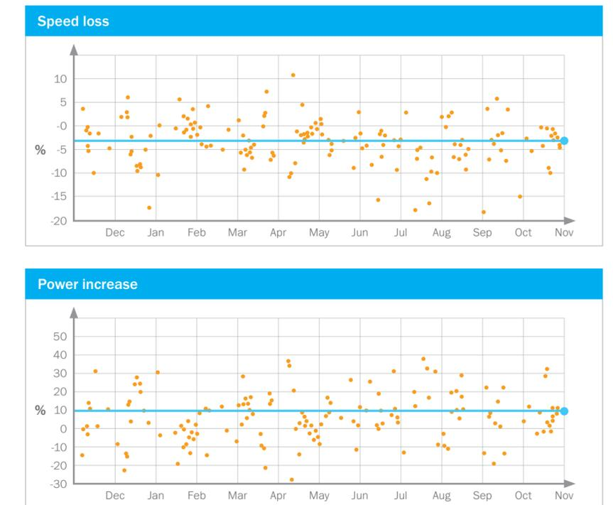
Figure 3: Actual speed loss values (upper) and power increase values (lower) for a 9300 TEU container vessel during a one-year period. Orange dots are data points while blue lines show average values during the period.
