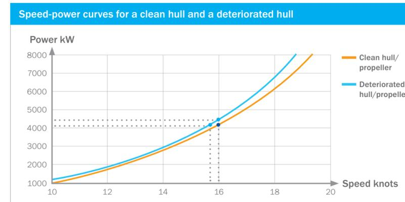
Figure 2: Illustration of changes in the speed-power relationship between a clean hull and a deteriorated hull.
