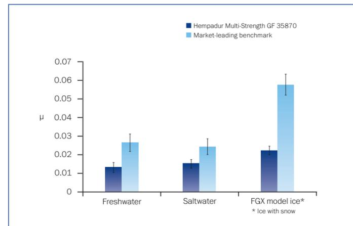
“Based on the test results, it seems that the friction of Hempadur Multi-Strength GF 35870 is lower than the friction of the reference paint in all ice conditions. The effect of the about 50 per cent decrease in friction is rather significant for ship performance, and should cause a decrease in the order of 5-15 per cent in total resistance of the ship in ice.”
