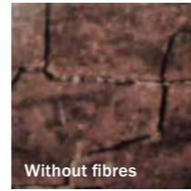
Coating condition after exposure to a cyclic blister box test: No failures were observed on the panel reinforced with microfibres. The coating without microfibres showed severe cracking.
