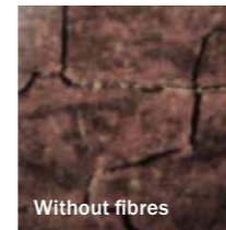
Coating condition after exposure to a cyclic blister box test: No failures were observed on the panel reinforced with microfibrils. The coating without microfibrils showed severe cracking.
