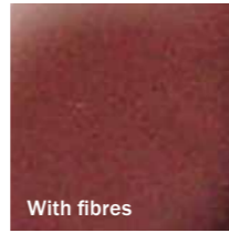
Coating condition after exposure to a cyclic blister box test: No failures were observed on the panel reinforced with microfibres. The coating without microfibres showed severe cracking.
