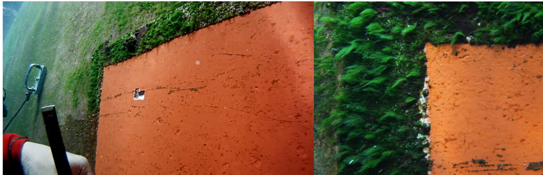
Figure 7: Pictures of a test patch mechanically damaged by scratches. The pictures were taken after 22 months in service.
