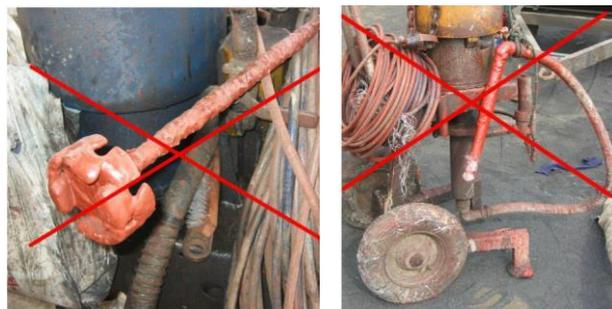
Figure 1. Non-acceptable condition of wet end of the suction pipe and stirrer. All components must be thoroughly clean prior to application
