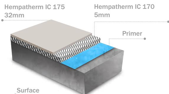
Application: Spray applied using low-pressure high-volume spray equipment.
