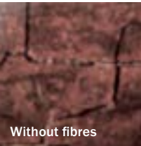
Coating condition after exposure to a cyclic blister box test: No failures were observed on the panel reinforced with microfibres. The coating without microfibres showed severe cracking.
