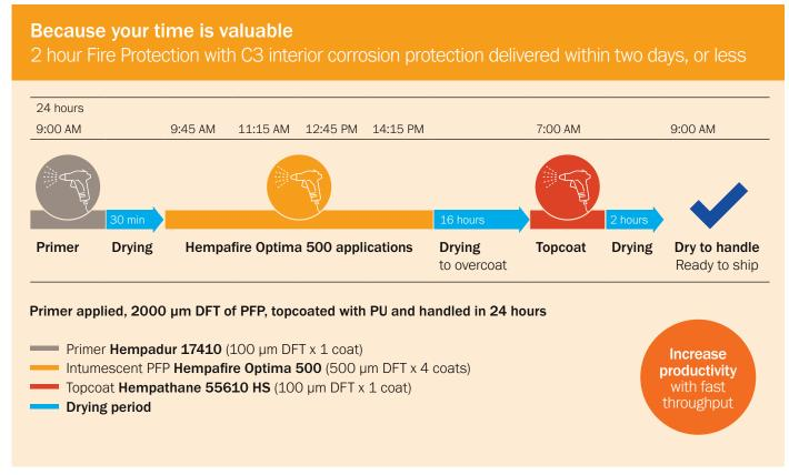
\*At 40°C and below 50 per cent relative humidity. Higher temperatures or lower humidity may reduce drying times and vice versa. Total drying times and PFP thicknesses may depend on your project specific conditions, application process and steel sections. Any steel section covered in our assessment can be potentially protected within 48 hours.
