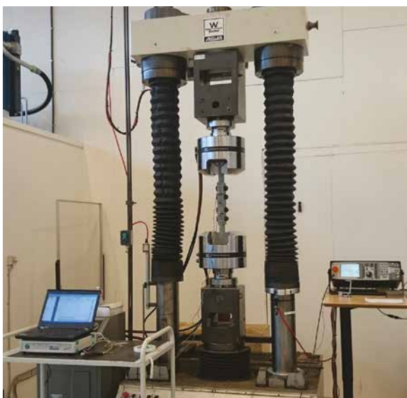
Figure 1. Amsler W Tester mounted with the test specimen
