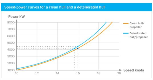
Figure 2: Illustration of changes in the speed-power relationship between a clean hull and a deteriorated hull.
