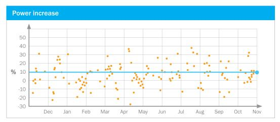
**Figure 3:** Actual speed loss values (upper) and power increase values (upper) for a 9300 TEU container vessel during a one-year period. Orange dots are data points while blue lines show average values during the period.
