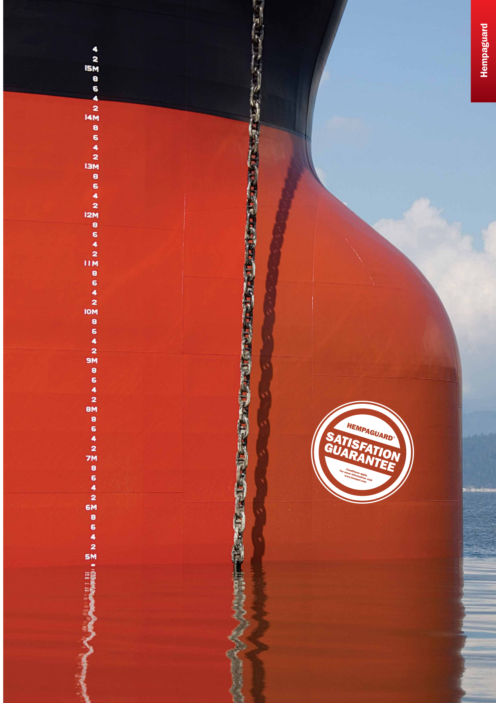
Upon immersion of the low-friction silicone coating, a hydrogel microlayer forms at the silicone-water interface where it acts as a physical fouling defence.
