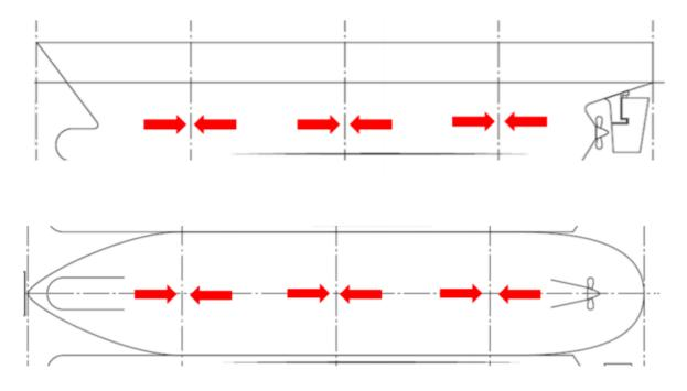
Figure 2: Example of recommended painting scheme for large structures to avoid exceeding maximum self-overcoating interval of Hempel's Nexus II (vertical sides and flat bottom)
