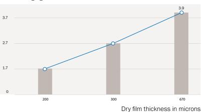
The graph shows that the increase of Contex EM thickness can bridge wider cracks.
