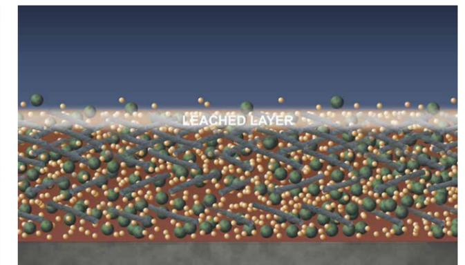
The antifouling coating after exposure to seawater. As a result of the biocide release, a leached layer starts to form. Water flow and the parallel structure of the fibres facilitates the smooth and uniform removal of the leached layer, ensuring a well-controlled polishing rate throughout the coating's entire service life.
