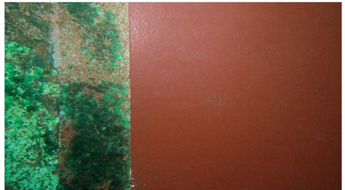
After 45 months, the Hempaguard test patch was inspected during a night dive in Singapore. The Hempaguard test patch was still smooth and fouling free. This 'remarkable' performance has convinced Euronav to complete full-scale Hempaguard applications on a number of vessels, starting with the Suezmax Devon.
