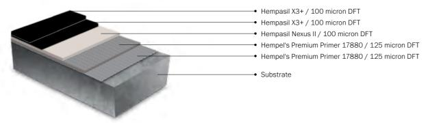
Converting from the existing antifouling system – 3 year scheme
