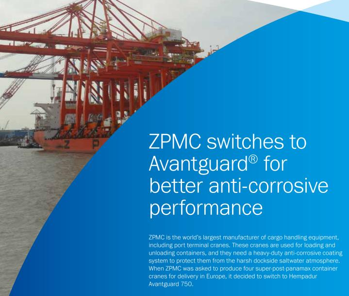
ZPMC had been using one of our zinc-rich epoxy primers to protect its cranes, and was pleased with the coating's performance. But only around one-third of the zinc in a traditional zinc epoxy has an anti-corrosive effect. Avantguard technology activates all of the zinc in the coating, which significantly improves the coating's anti-corrosive performance and mechanical strength, while ensuring it remains easy
