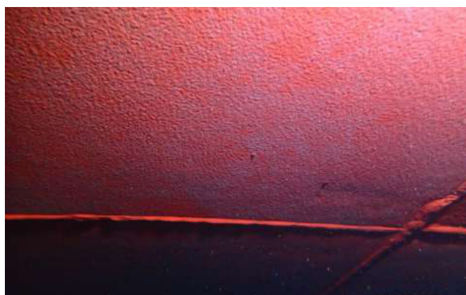
Photos from the in-water hull inspection showed that verticals and flat bottom were clean
