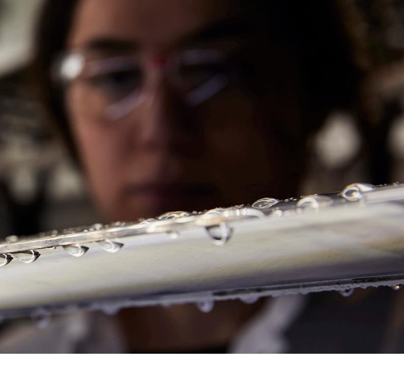
At Hempel, we have our own in-house DNV GL RP-0171 compliant RET facility. And we've put Hempablade Edge 171 to the test in more than 500 exhaustive test sessions and assessments. This not only ensured the optimisation of its development and the LEP validation process, but it also means you can be sure it is proven to protect against rain erosion
